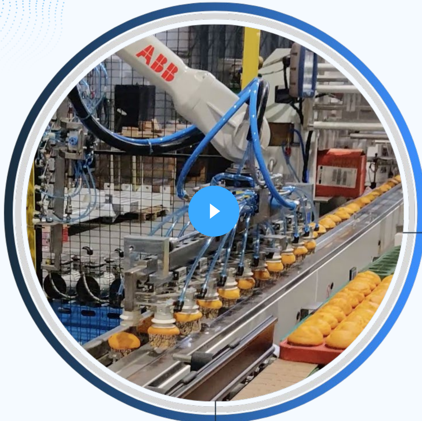
End-of-line automation Vacuum gripper for muffin handling
